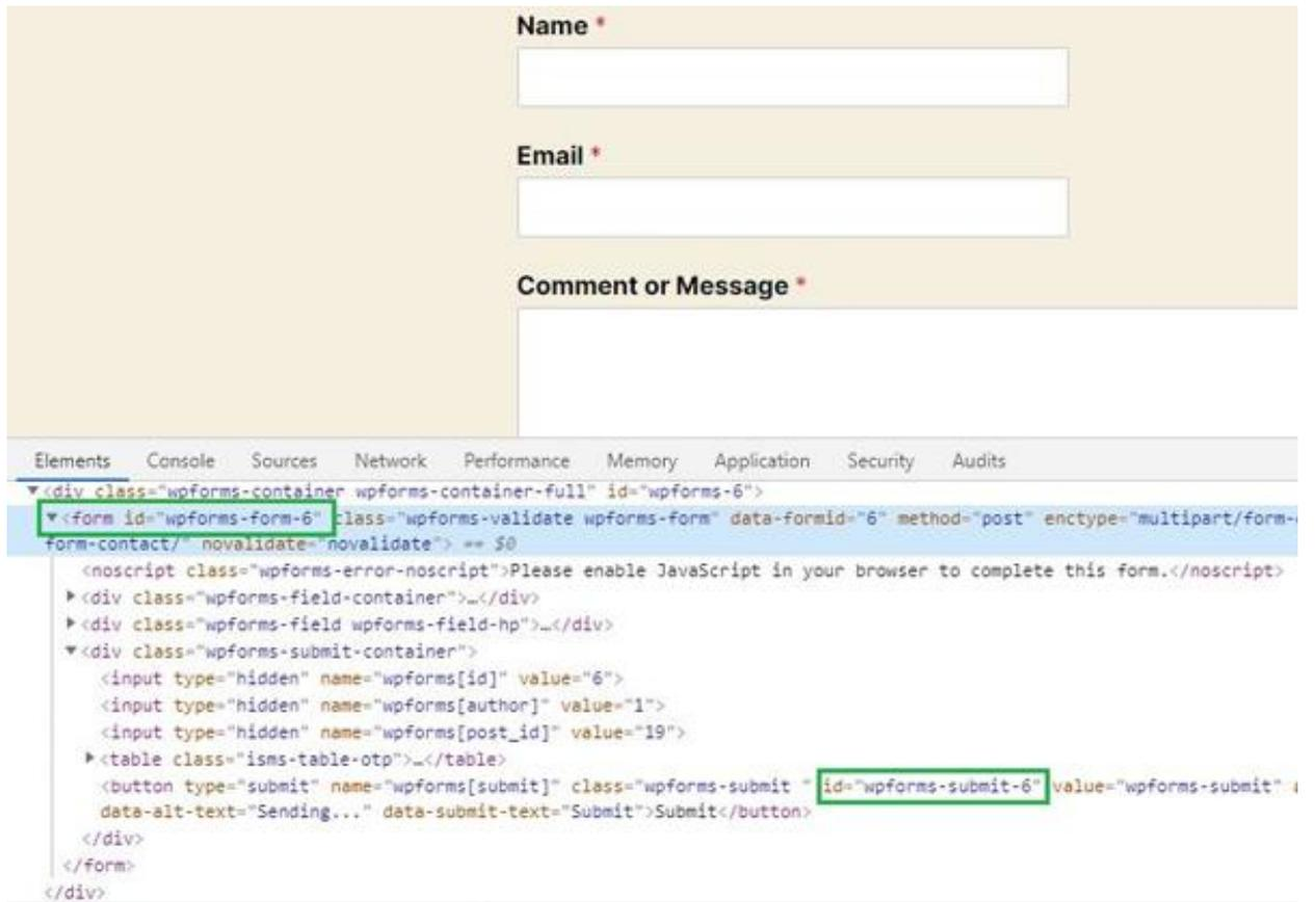
The image shows a contact form with three input fields: "Name \*", "Email \*", and "Comment or Message \*". Below the form is the Chrome DevTools "Elements" panel. The selected element is the form container, and its HTML structure is displayed. Two specific attributes are highlighted with green boxes: the form's ID, "wpforms-form-6", and the submit button's ID, "wpforms-submit-6".
